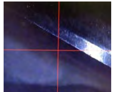
An example of a carbide cutting tool with no wear.
