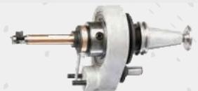
**Air or Coolant Style Autofacer:** Is activated with thru-spindle coolant or air pressure to open the blade. Spring pressure in the clutch will close the blade when thru-spindle coolant is turned off.
