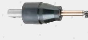
**Bump or Cone Style Autofacer:** Spring loaded tapered cone grips the face of the work piece to open and close the blade.
